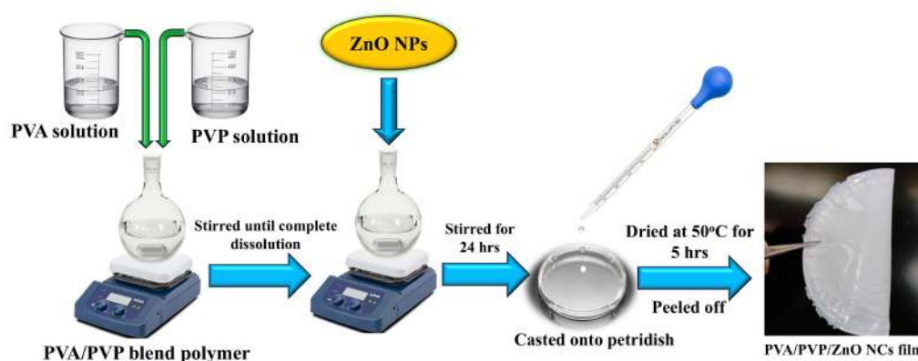
Figure 1: Schematic representation for the preparation of PVA/PVP/ZnO nanocomposites.
